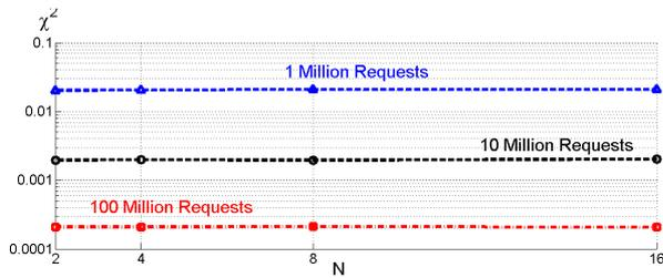
Figure 5:  $\chi^2$  analysis of an implementation of D-Zipfian generating requests. This analysis compares centralized Zipfian’s probability for different data items with D-Zipfian as a function of different degrees of parallelism (x-axis).  $M=10,000$ ,  $\theta=0.27$ .
